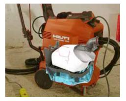
One filter bag recycles waste water up to 7 times which equals up to 100 litres of water output
